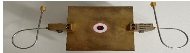
Fig. 1. RuDR test-fixture designed by EM modeling: ruby cylinder in the center, mounted with a Teflon ring (white) in a metallic enclosure. Copper foils will be placed as top and bottom of the resonator.
