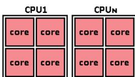
**QW-OMP:** this version uses OpenMP programming standard to accelerate preprocessing and FDTD loop. Because of high parallel efficiency and no changes in the project required in comparison to standard version, the QW-OMP can become the main *QW-MultiSim* version. QWED recommends using this version as a very convenient, easy and efficient tool for speeding up preprocessing and FDTD calculations.
