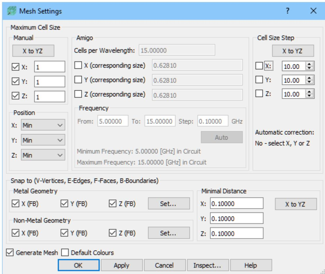
We set 1mm cell sizes in X, Y and Z direction. The meshing will be enforced in the entire project space.
