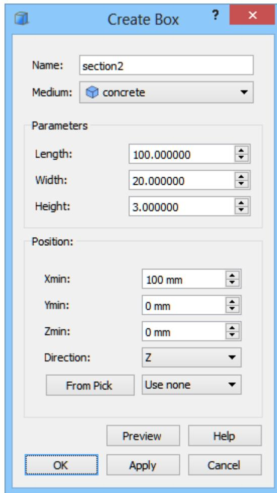
The name of this part is set to “section2” and its medium is chosen to be *concrete*. The dimensions of this part are the same as in the case of air filled section. The concrete filled part is placed behind the *section1* thus its position in X direction is set to 100 mm. After pressing *OK* button the concrete filled part of the transmission line appears in the project.
