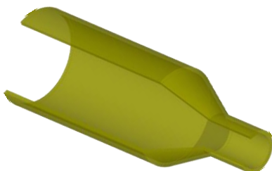
Coaxial structure used as an output of a travelling wave tube (TWT).
