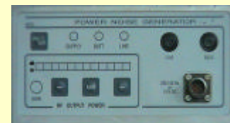
L(1.2-1.4GHz), S(3-3.5GHz), C(5.3-5.9GHz) - Band Noise Sources (NS)
