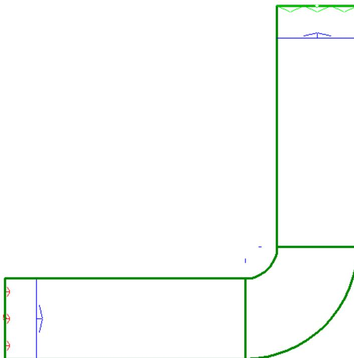
Fig. 1 Scheme of E-plane WR-10 waveguide bend proposed in [1].
