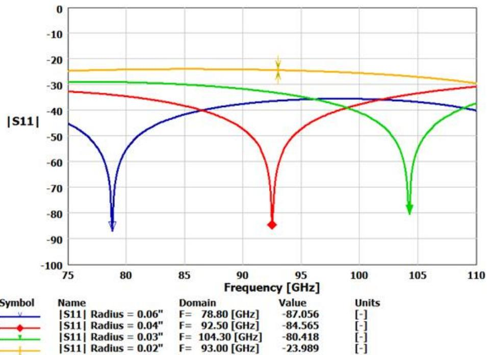
Fig. 3 Magnitude of reflection coefficient of E-plane bend for different values of the inner radius, computed with QuickWave 3D.
