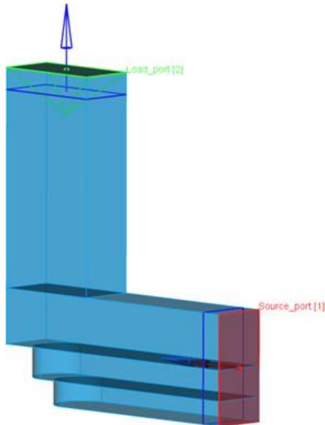
**Fig. 6** Simulation model of H-plane WR-10 waveguide bend, prepared in QW-Modeller [3].
