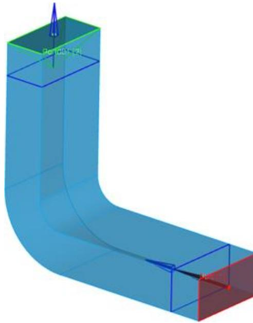
Fig. 2 Simulation model of E-plane WR-10 waveguide bend, prepared in QW-Modeller [3].
