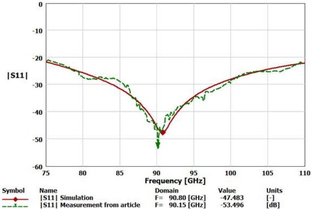
Fig. 9 The magnitude of reflection  $|S_{11}|$  coefficient of H-plane bend – simulated data and measurements from [1].
