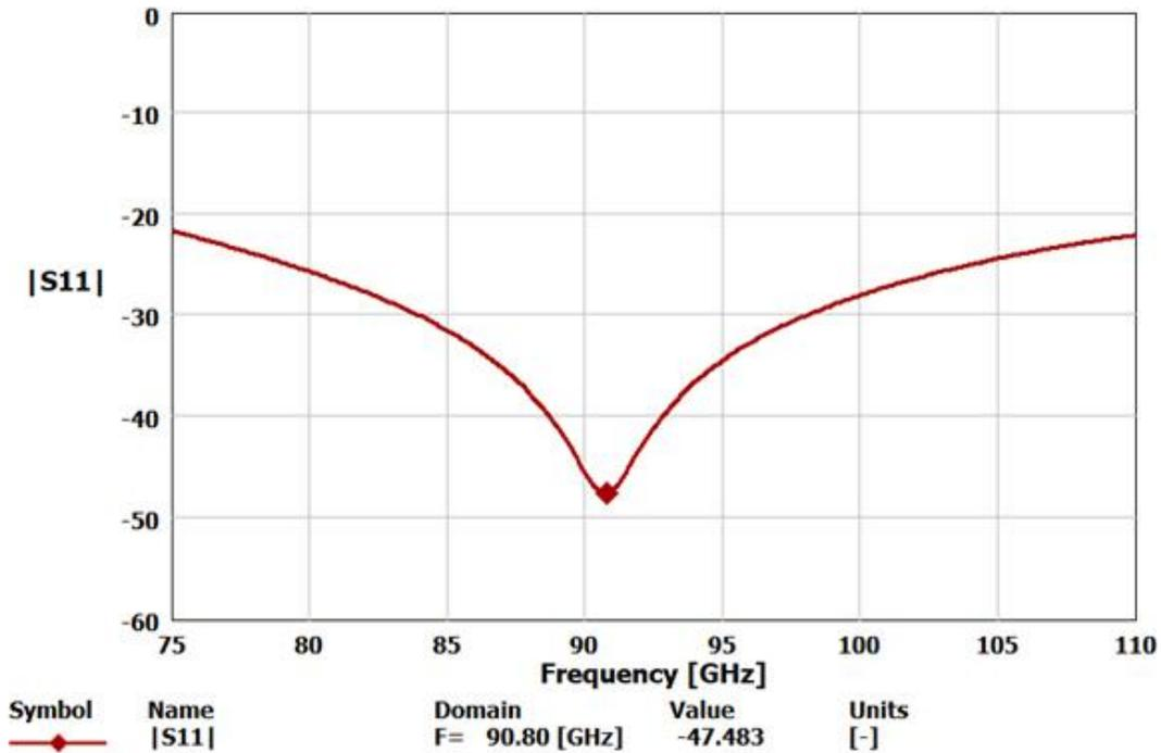
Fig. 7 Magnitude of reflection coefficient of H-plane bend computed with QuickWave 3D.
