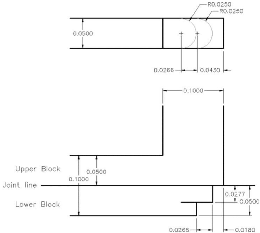
**Fig. 5** Scheme of H-plane waveguide bend proposed in [1]. All dimensions are given in inches.
